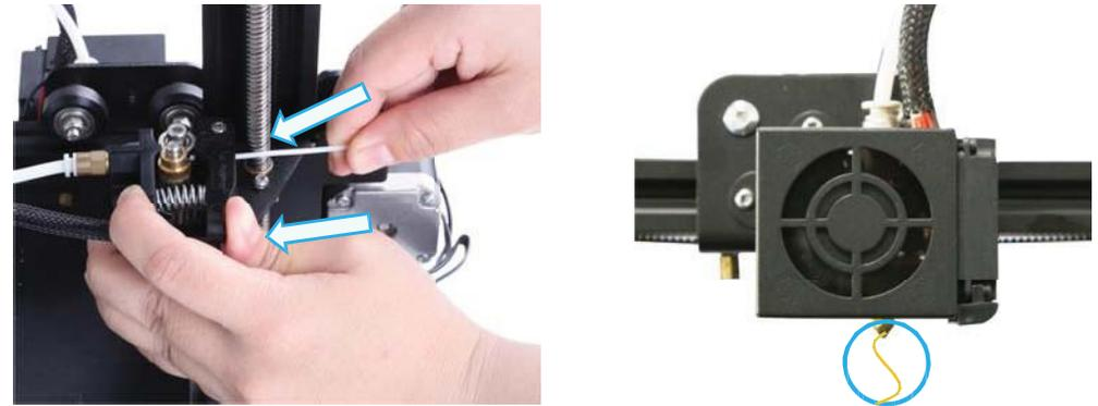
Press and hold the extruder lever then insert 1.75mm filament through the small hole of the extruder. Continue feeding until you see filament come out the nozzle.
